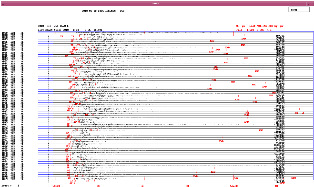
Figure 32: Plotting the automatic phase reading with waveforms.
