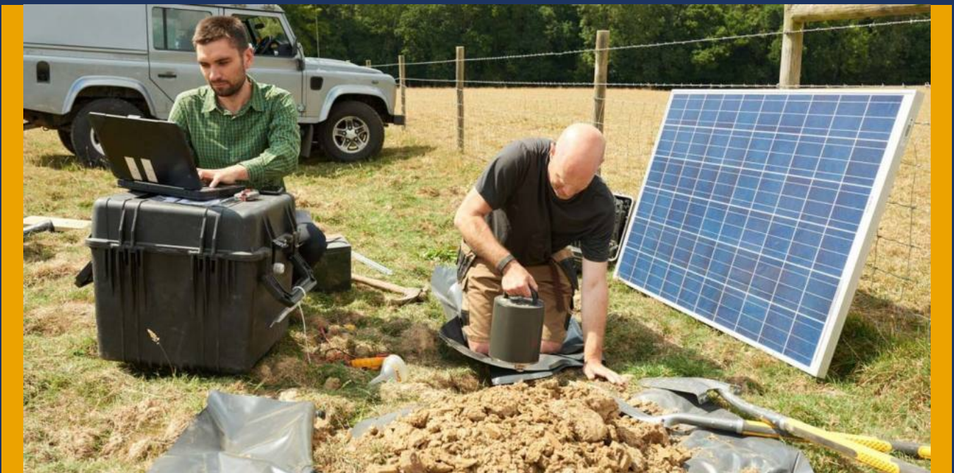
Image 1: Seismometer installation in the field to monitor for earthquakes. This is an important part of establishing natural baseline conditions and can identify impacts of human activity in the subsurface. Credit: BGS © UKRI
