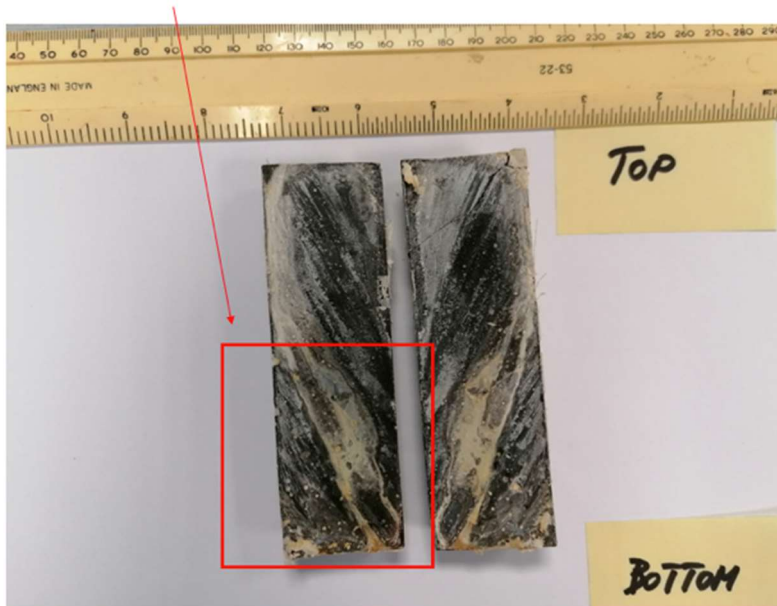
Figure 14. Reacted cement core split open along the cut surface, and showing light-coloured precipitates.
