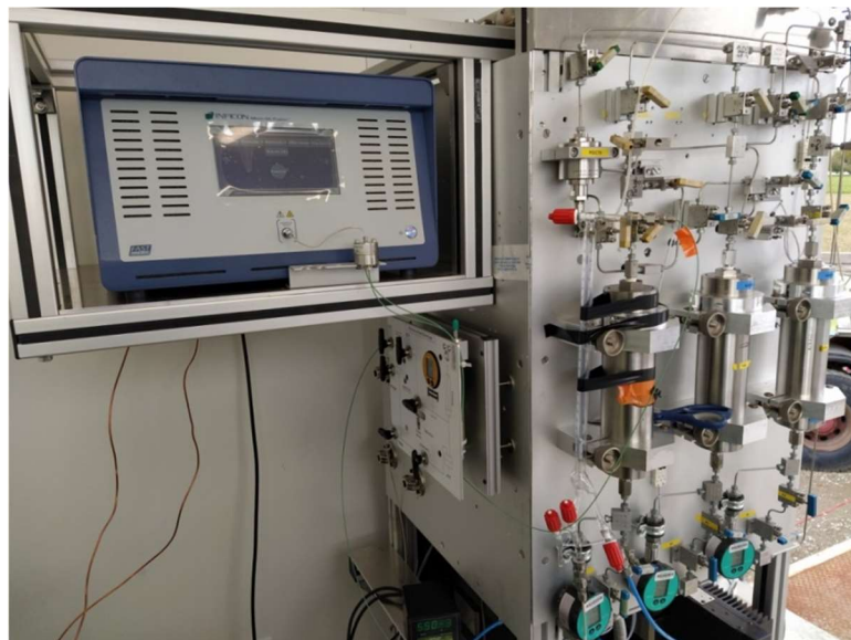
Figure 7: Custom glass burette and optimized dead volumes between burette and \mu -GC
