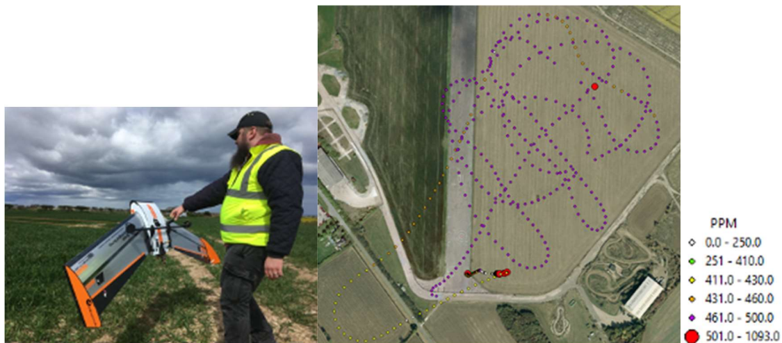
Figure 1. BGS fixed-wing UAV CH 4 sensor prototype (left) with results plotted from a UK test flight (right)
