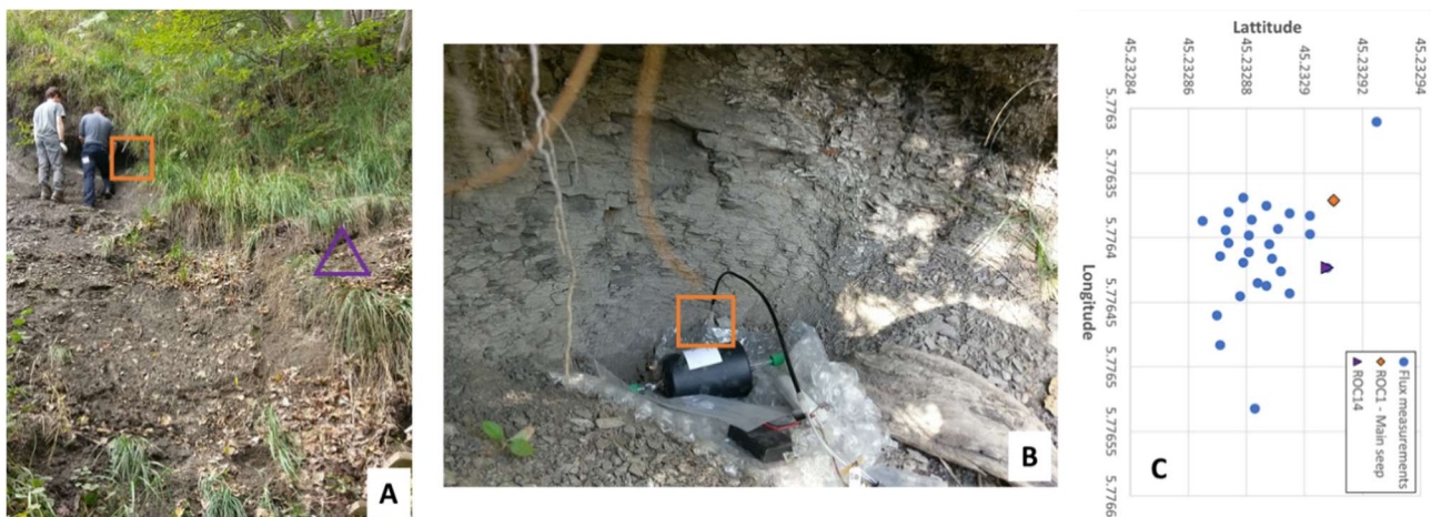
Figure 2: A. Rochasson (ROC) sampling site. Orange square=sample ROC 1 (main vent), purple triangle=sample ROC14 (soil sample). See Figure 1A for location of the Rochasson site. B. Sampling equipment at the main vent (ROC1). C. Soil flux measurements (blue dots) with location of the collected gas samples (see SECURE Report D3.4, 2021 for results). Note that map is rotated 90° to align with photo in A.
