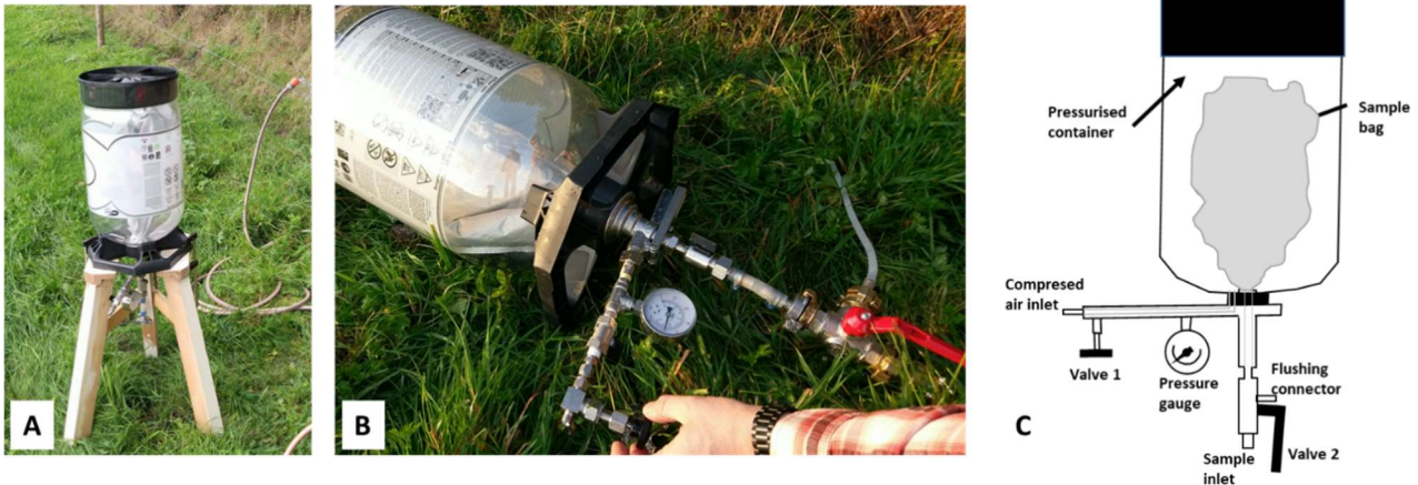
Figure 7: A. Photo of the double walled sampling container with the sampling bag. B. Detailed photo of the sampling valves. C. Schematic drawing of the sampling setup. Compressed air inlet is used to pressurise the container with valve 1 and pressure gauge for depressurisation. Sample inlet is connected to the pumps collecting the groundwater and has a second valve that allows to flush sampling valves prior to sample collection.
