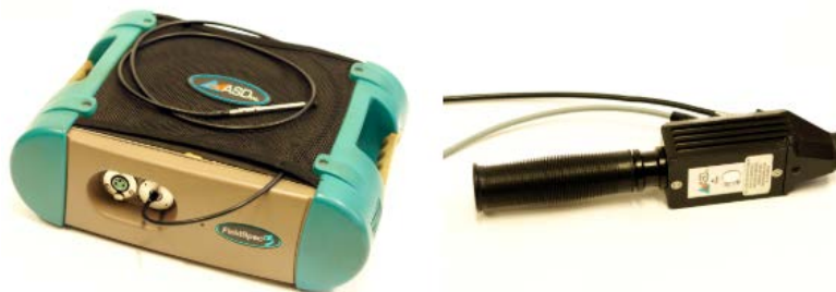
Figure 19 Spectroradiometer ASD Panalytical for hyperspectral signature acquisition onsite (source: nerc.ac.uk)
