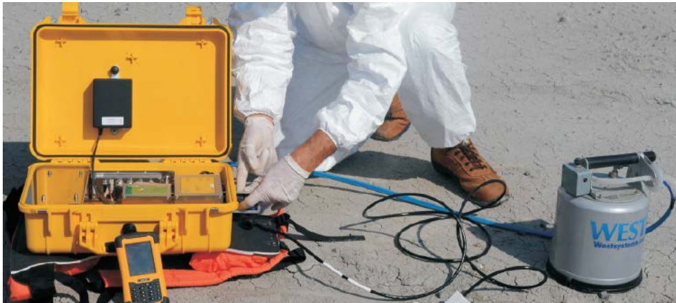
Figure 18 Accumulation chamber West Systems for CH 4 , CO 2 , VOC and H 2 S fluxes measurement onsite at soil/atmosphere interface (source: westsystems.com)
