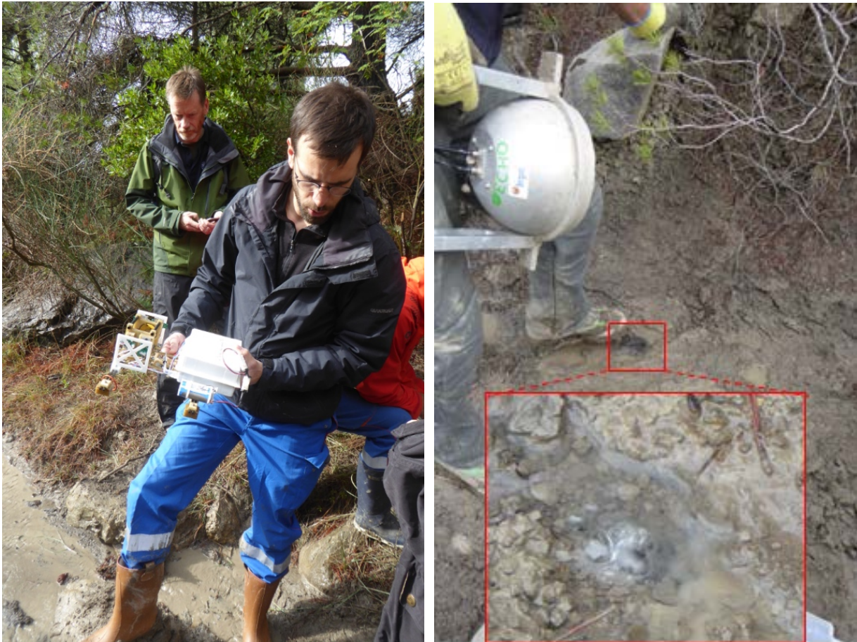
Figure 8 AUSEA sensor in operation at Jonchiers (left). View of the CH 4 emission point discovered in 2019 (right).
