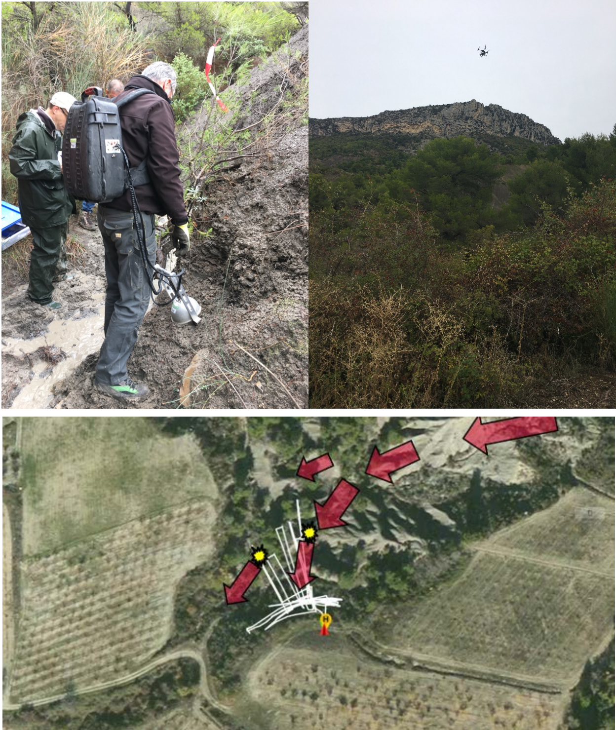
Figure 6 In-situ gas flux measurements by BRGM (top left). TOTAL AUSEA UAV sensor combining CO 2 and CH 4 drone-based sensor deployed by TOTAL at Jonchiers (top right). Plot of a selection of flight paths (while lines) with prevailing wind direction (red arrows) and take-off spot (H) (bottom).
