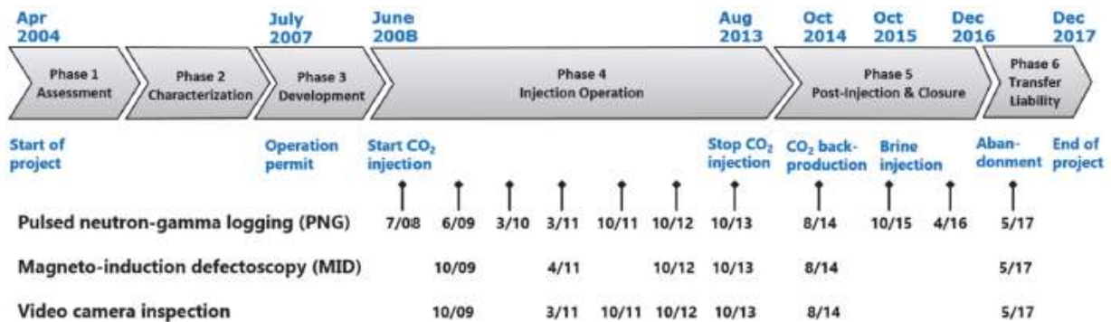
Figure 2 Post-injection well integrity monitoring (month/year) with the completed storage cycle of the Ketzin CO 2 storage site from (Schmidt-Hattenberger et al., 2018)
