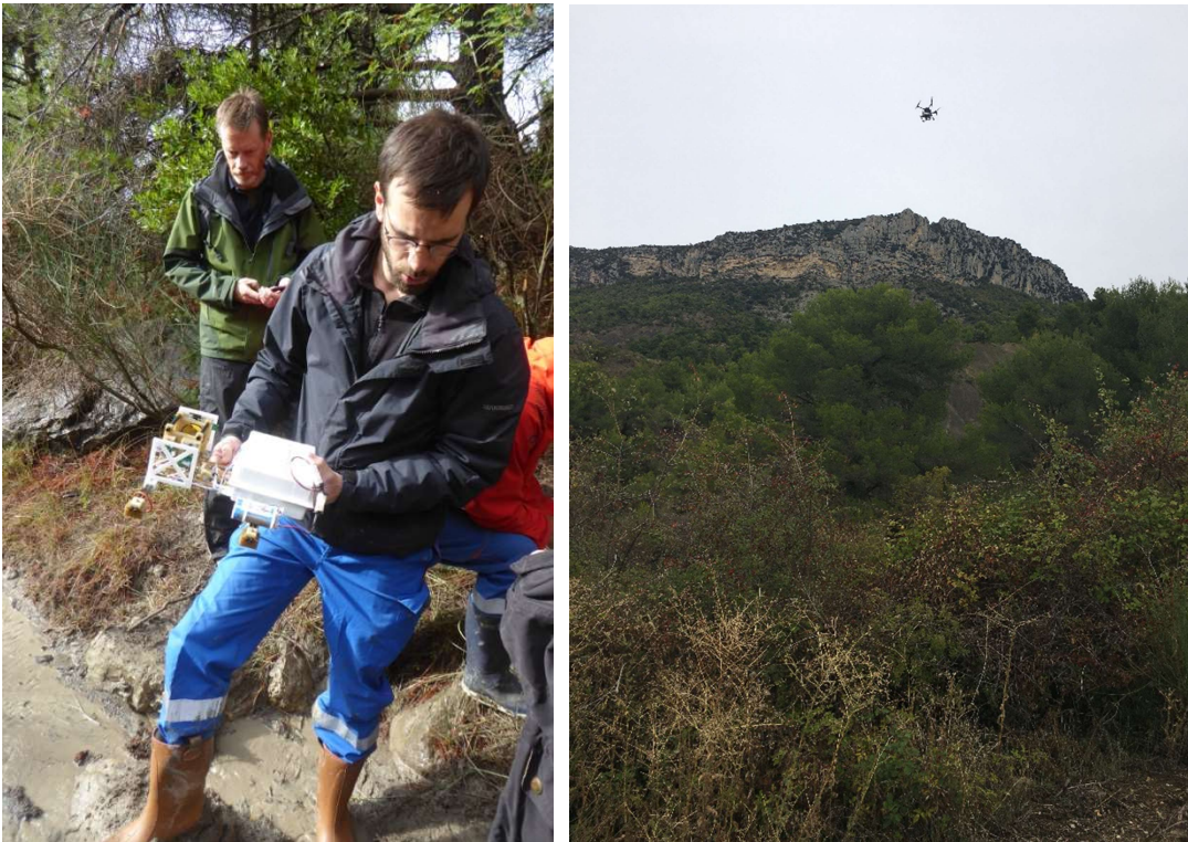
Figure 2 October 2019 fieldwork at French Alps natural gas seeps. Left: Walkover survey with the TOTAL gas sensor. Right: Gas sensor flown on a rotary drone
