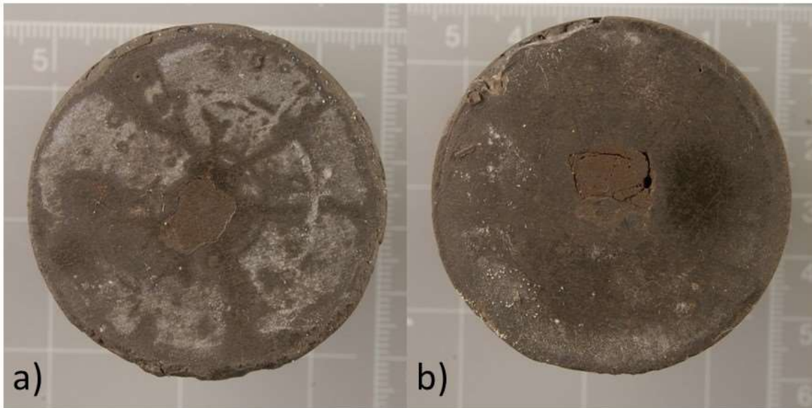
Figure 10 Post-test pictures of samples with Low-density Portland G (a) and Flexible Portland G (b) as sealant material.
