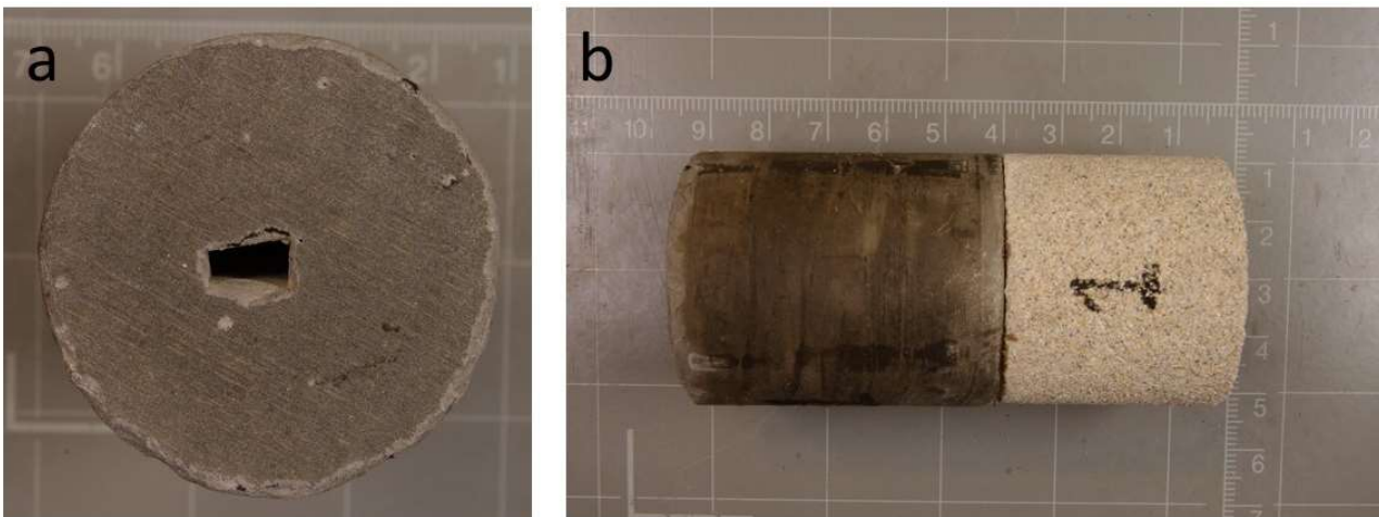
Figure 2 Pictures of the prepared slit before sealant material is injected (a) and the cement- Castlegate sample (b).
