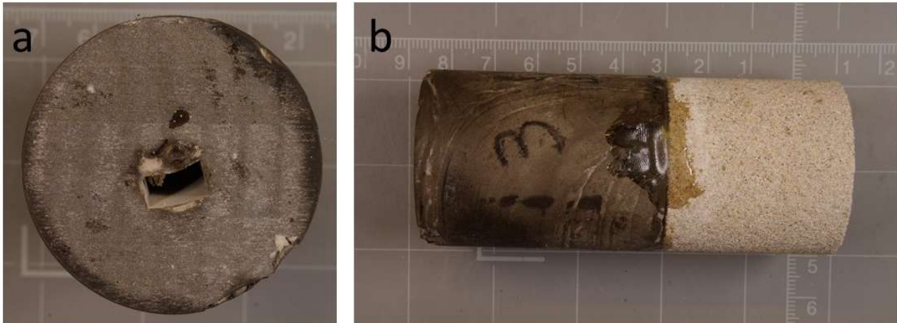
Figure 3 Pictures of the manufactured slit before sealant material is injected (a) and the cement-Castlegate sample (b).
