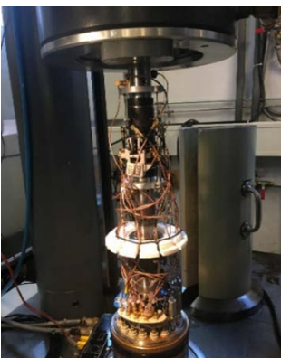
Figure 1. Instrumentation around a sleeved core plug (deformation gauges and ultrasonic transducers).
