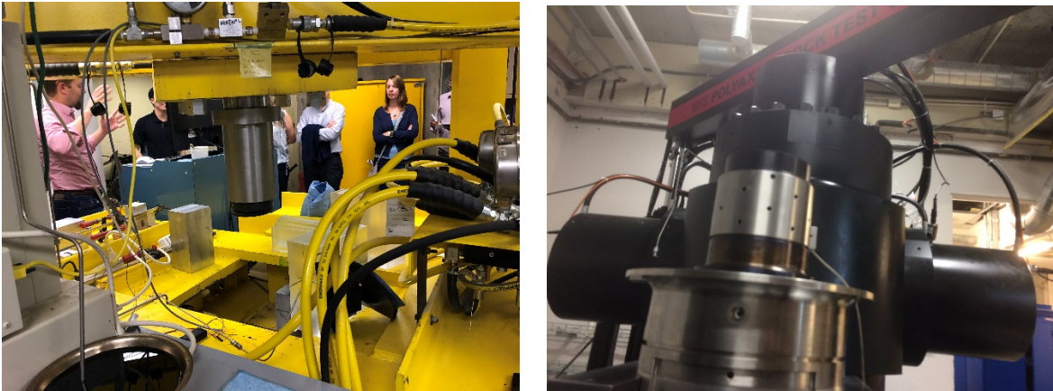
Figure 3. True triaxial load frames allowing for 3 different applied stress components. Left: University of Pittsburgh; right: SINTEF.
