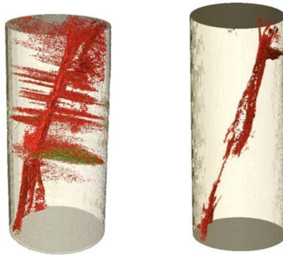
Figure 10. Micro-CT image reconstruction isolating the fracture planes detected in the two sandstone specimens with stress-induced fractures. Left: Mt. Simon sandstone; right: Castlegate sandstone (Cerasi et al. , 2018).
