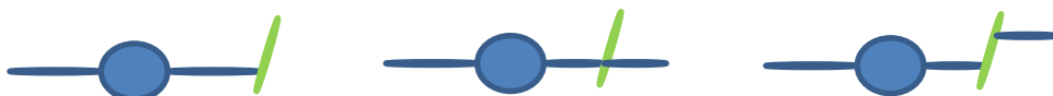
Figure 4. Three different possible interactions between a hydraulic fracture (in blue) from an injection well (oval) and a natural fracture (green) in its vicinity. Left: the triggered fracture is arrested by the natural fracture (inflating it or possibly reactivating it); middle: the triggered fracture traverses the natural fracture; right: the triggered fracture is deviated by the natural fracture.
